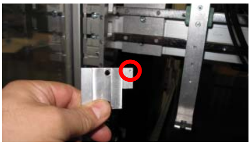
Remove the 30mm fingers.
