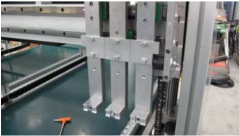
Check that the side plates rest against the rubber stoppers as shown.
