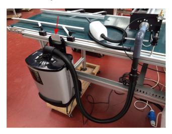
If you have the latest type drum seeder, disconnect the vacuum pump, and plug in the new vacuum. If you have the old drum seeder (green conveyor) remove the vacuum plug and connect to a separate electrical outlet with a suitable plug.
